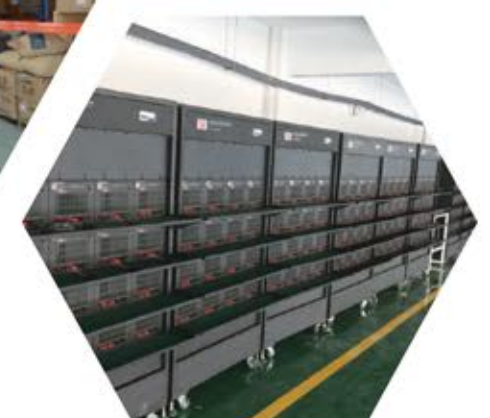
Lithium battery pack aging test machine
